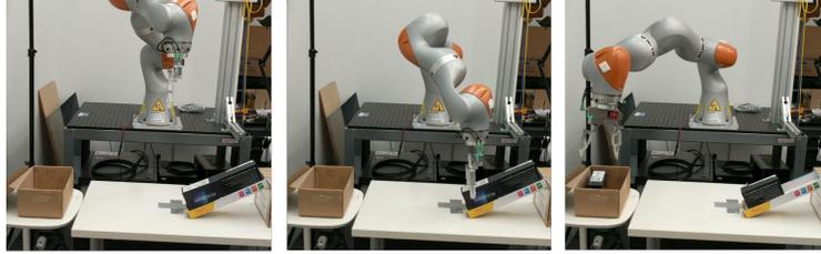
(a) A robotic arm picking objects and placing them in a bin. The robot learns how to accomplish the task from a single human demonstration by solving an SDP. See chapter 7 for more details.
